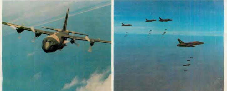
TOP: Firing at rate of 6,000 rpm each, miniguns on AC-47 aircraft strafe Viet Cong positions in South Vietnam. ABOVE LEFT: AC-130 — or Gunship II — carries high-intensity light, flares for battlefield illumination, advanced detection devices, four miniguns and four M-61 Vulcan 20mm cannons. ABOVE RIGHT: U.S. Air Force F-105s of 34th Tactical Fighter Squadron, 388th Tactical Fighter Wing, drop 750-lb. bombs on target during Combat Sky Spot Mission in Southeast Asia. Photos: USAF
